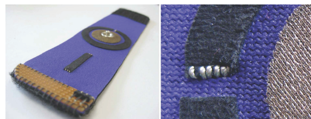
Fig.8 a,b) Time Sensing Bracelet and close-up of materials used for the resistive track and conductive center
